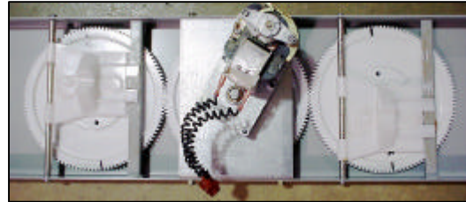
Figure 2 - Spur Gear Meshing Relationship (Bottom View of Top Cover)
