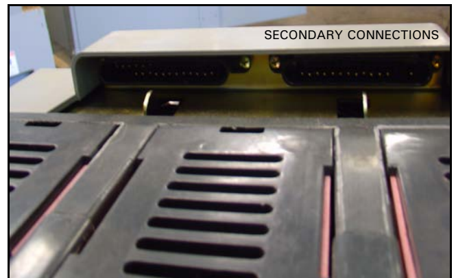
Figure 10. Primary and Secondary Connections on a Magnum Fixed Switching Device.
