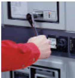
Magnum DS Breakers can be conveniently levered into the connect, test and disconnect positions without opening the breaker compartment door. Three faceplate indicators identify the positions by color.
